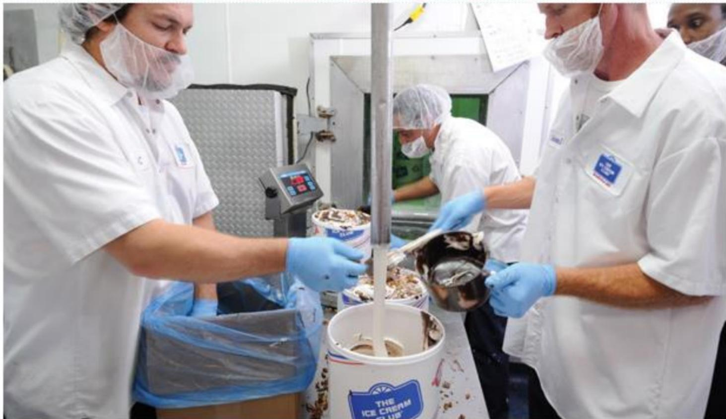
As ice cream flows from the freezer into a 3-gallon tub, Jim Cummins (left) and Coleman Kelleher add nuts and fudge sauce. Ricardo Santiago sends cartons into the blast freezer.
