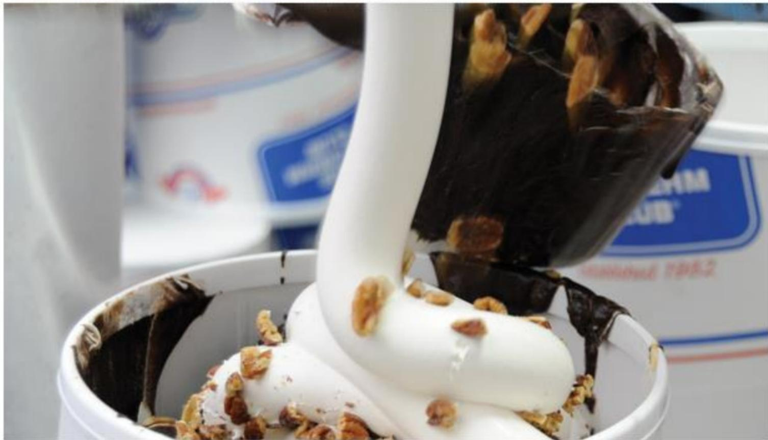
After a tub is filled, a lid is added and the carton will be weighed before it's conveyed to a hardening room.
